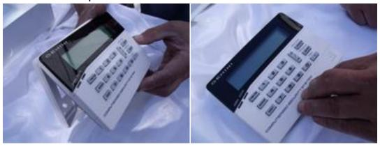
7. Run wire from keypad to control panel enclosure thru top grommet. You may cut off any excess wire and restripe ends. Connect wires by color codes in picture.
