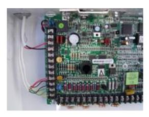
12. Make sure that switch on side of control panel enclosure is OFF. Connect preinstalled wire from switch (white terminal block) to your DC battery power. <u>POLARITY MUST BE CORRECT</u> RED(+) and BLACK(-) or you could <u>DAMAGE</u> control panel. Note: If your vehicle wiring is White & Black than the Black is probably (+) and White (-). Best to check with a volt meter.
