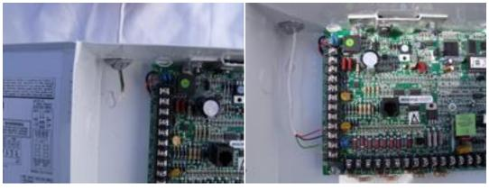
8. Mount wireless receiver with Velcro or long screws thru mounting holes on side of receiver. It can be mounted horizontal or vertical. Make sure that antennas are extended as pictured below.
