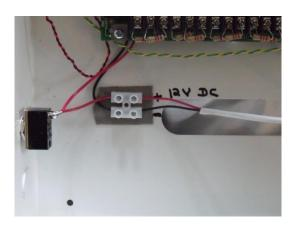
13. Turn control panel battery switch ON (Left side of Panel). If keypad shows trouble, than press RESET button on keypad. You're now ready to install the wireless devices.
