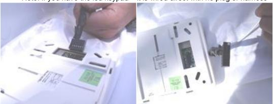
6. Hook keypad on top hinges of base plate. While pushing down on keypad, snap both bottom clasps.
